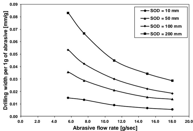
Fig. 4 Unit mass of abrasive effect on the drilling width
