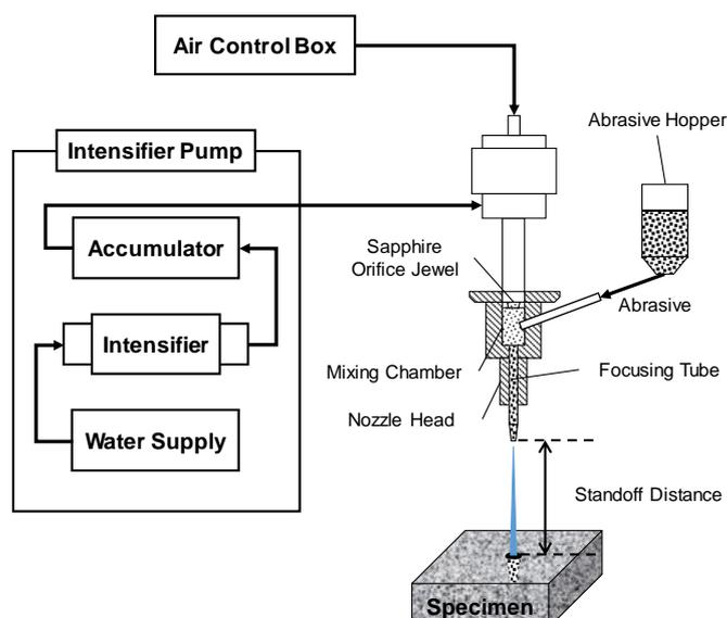
**Fig. 1** Abrasive waterjet system
