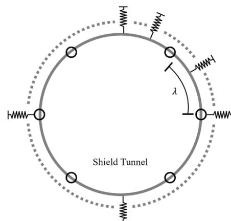
Fig. 2 Variation range of lining degradation
