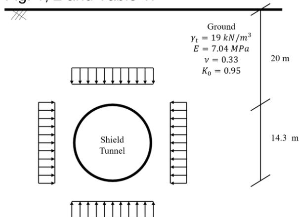
Fig. 1 Numerical model condition
