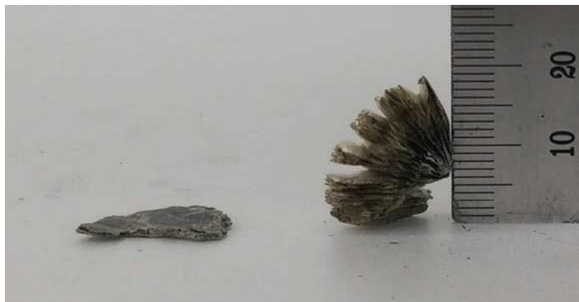
Fig. 1 Expansion of vermiculite by thermal energy (Ahn and Hu 2016)
