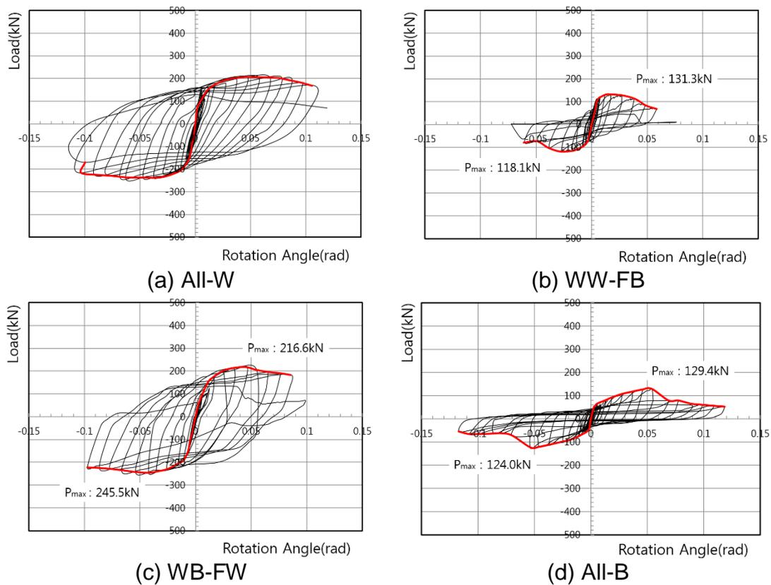
Fig. 4 Applied load vs. rotation relationship
