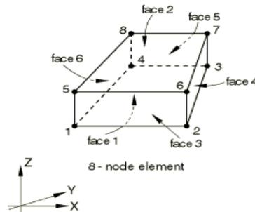
Figure 1 - solid element used for masonry blocks
