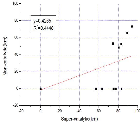
Fig. 6 Comparison of super-catalytic effect and non-catalytic effect for demise altitude
