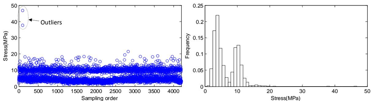
Fig. 7 Extracted peak stress sequences and stress histogram
