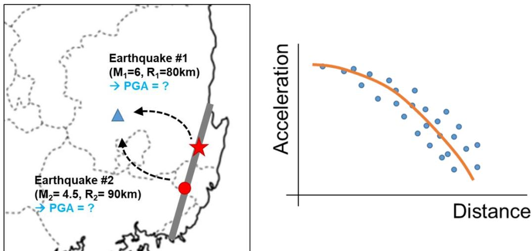
Fig. 1 Prediction of ground motions with respect to earthquake magnitude and epicentral distance
