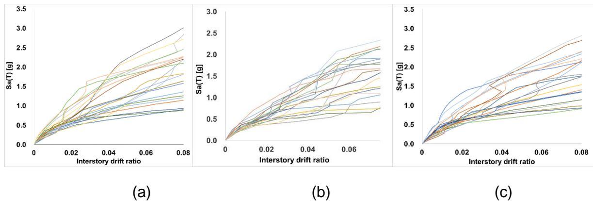
Fig.3. IDA curves for 3 models: (a) Model A; (b) Model B; (c) Model C
