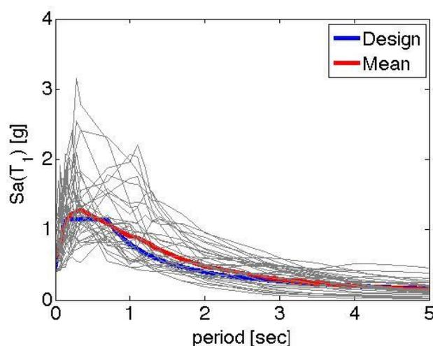
**Fig. 2.** Spectra of ground motions used in the simulations
