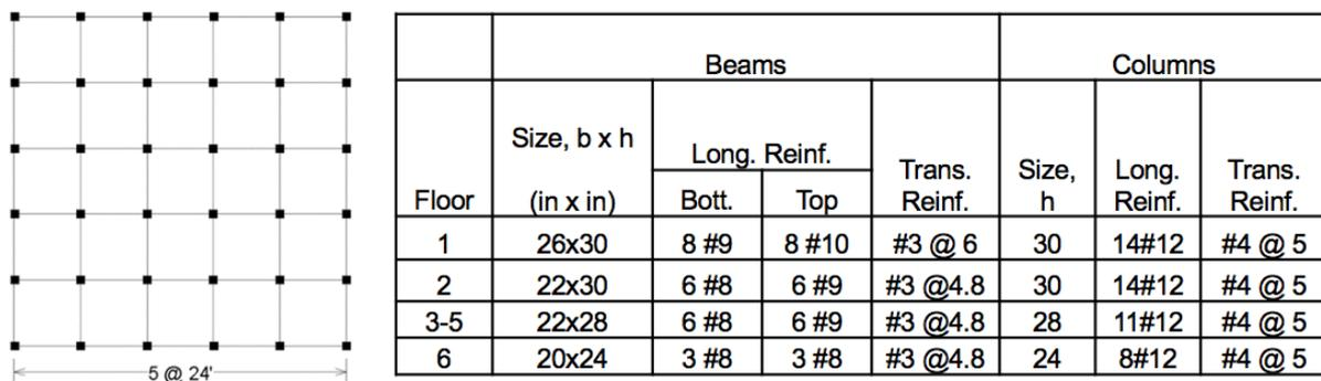
**Fig.1** Plan view of the 6-story RC frame building with section and reinforcement details
