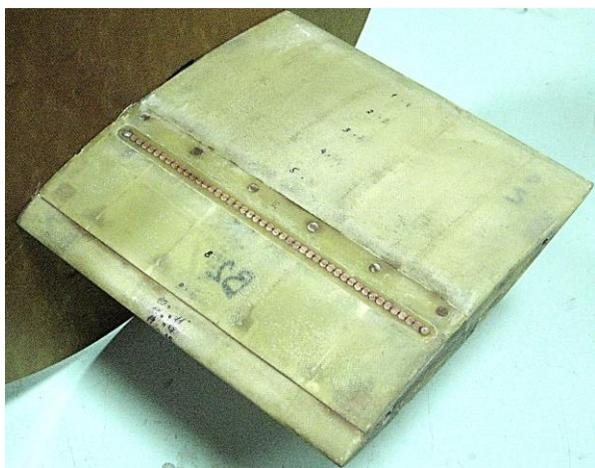
Fig. 4. Airfoil (SAP) model contours (top) and mounted spark plasma insert (bottom): 1 - left endplate; 2 - discharge gaps; 3 – pressure taps; 4 – plasma array insert.
