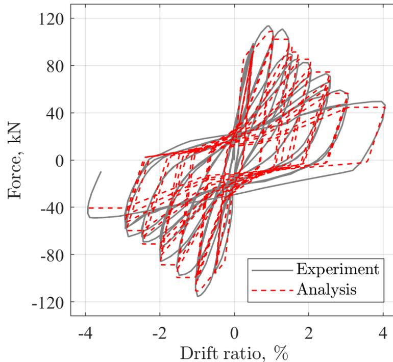
**Fig. 2** Force-deformation response of experiment and analysis
