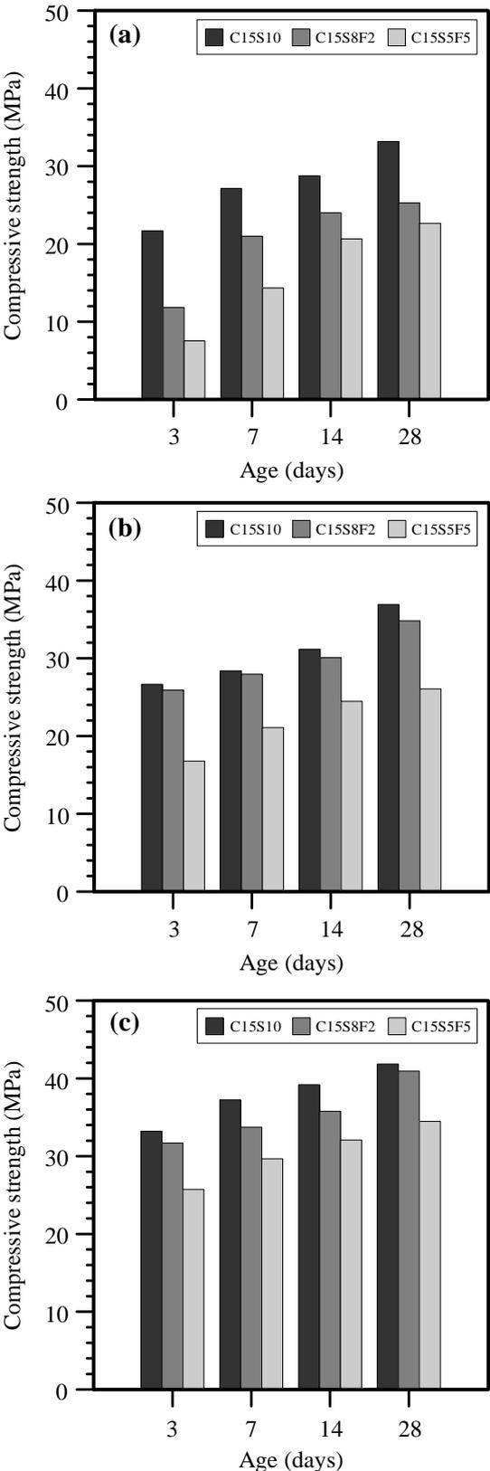
Fig. 2 Strengths development of hardened paste with different curing schemes: (a) T20, (b) T30 and (c) T40
