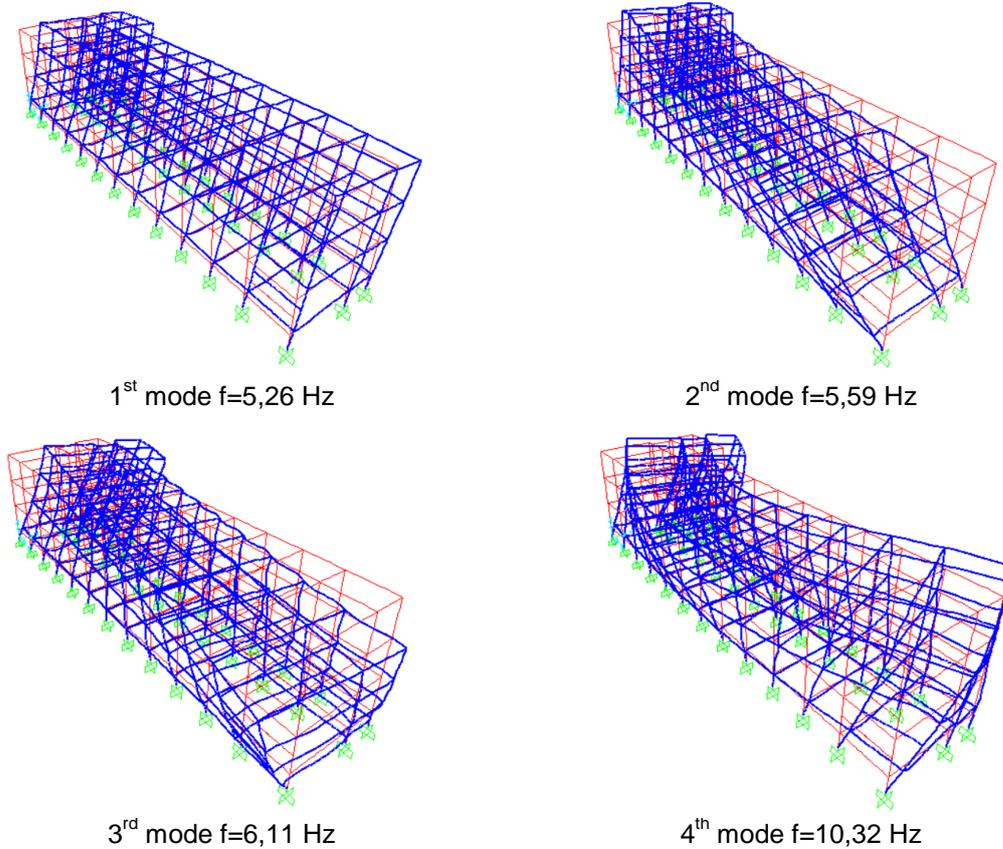
**Fig. 9** Modal shapes obtained with f.e. model before retrofitting
