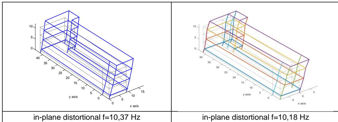
Fig. 4 Modal shapes before and after retrofitting
