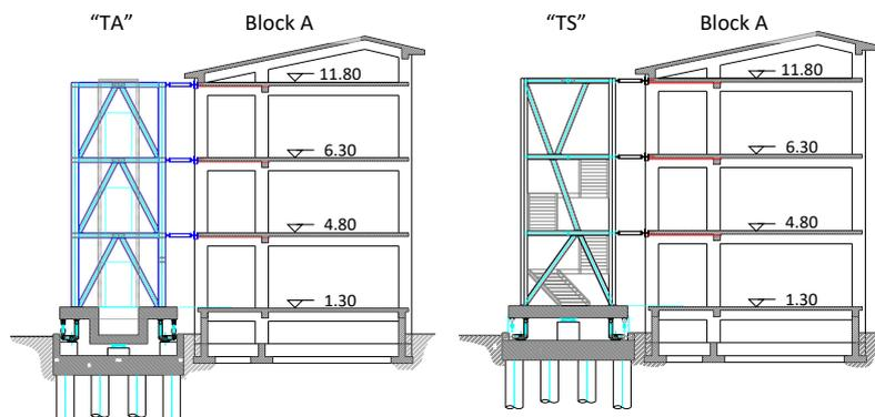
Fig. 2 Sectional elevations of block A with dissipative towers in the transverse direction
