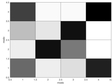
Fig. 6 MAC Matrix between modal shape obtained before and after retrofitting
