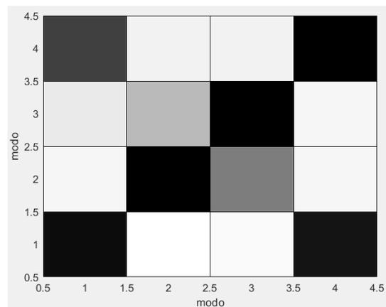
**Fig. 10** MAC matrix of the modal displacements obtained with the experimental tests and with the f.e. model before retrofitting
