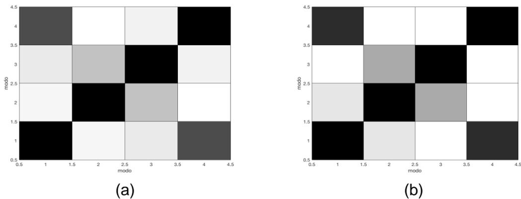
Fig. 5 AutoMAC Matrix: (a) Before Retrofitting; (b) After Retrofitting
