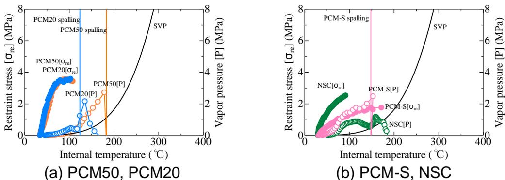
Fig. 10 Internal temperature, restraint stress, and vapor pressure at 40 mm
