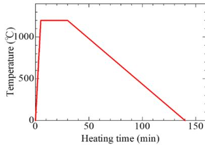
Fig. 2 RABT30 rapid heating curve
