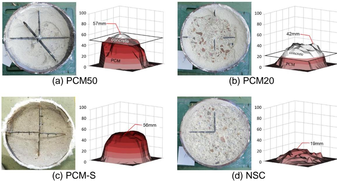
Fig. 4 Results of the heating surface and spalling depth contours
