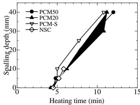
Fig. 5 Temporal changes in the spalling depth
