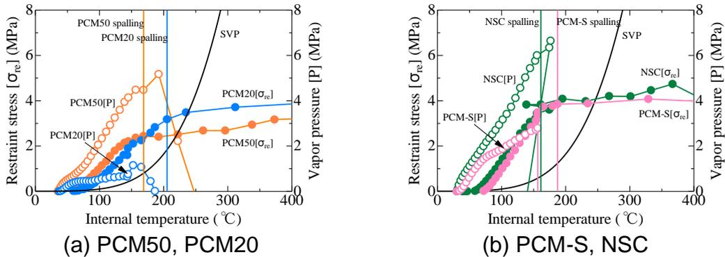
Fig. 9 Internal temperature, restraint stress, and vapor pressure at 5 mm
