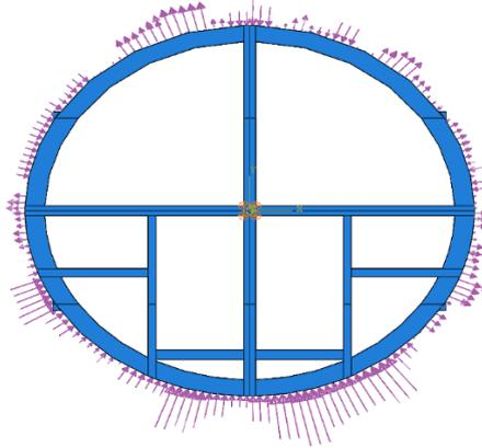
**Fig. 1** Equivalent static irregular wave pressure distribution
