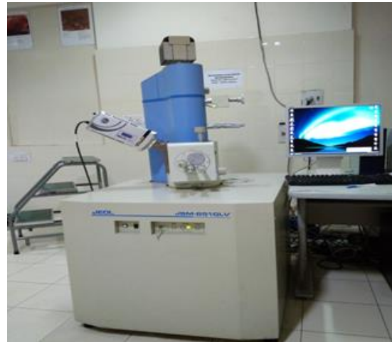
Fig.3. Set-up for microstructural characterization (a) Gold etching machine, (b) SEM analyzer.
