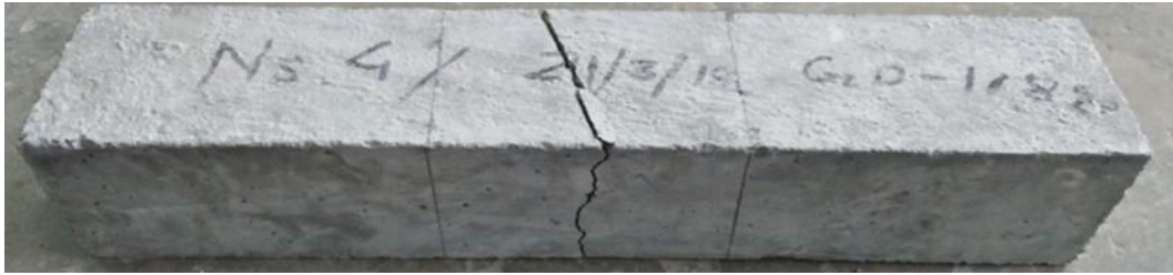
Fig. 2. Prism showing crack pattern after flexural testing.
