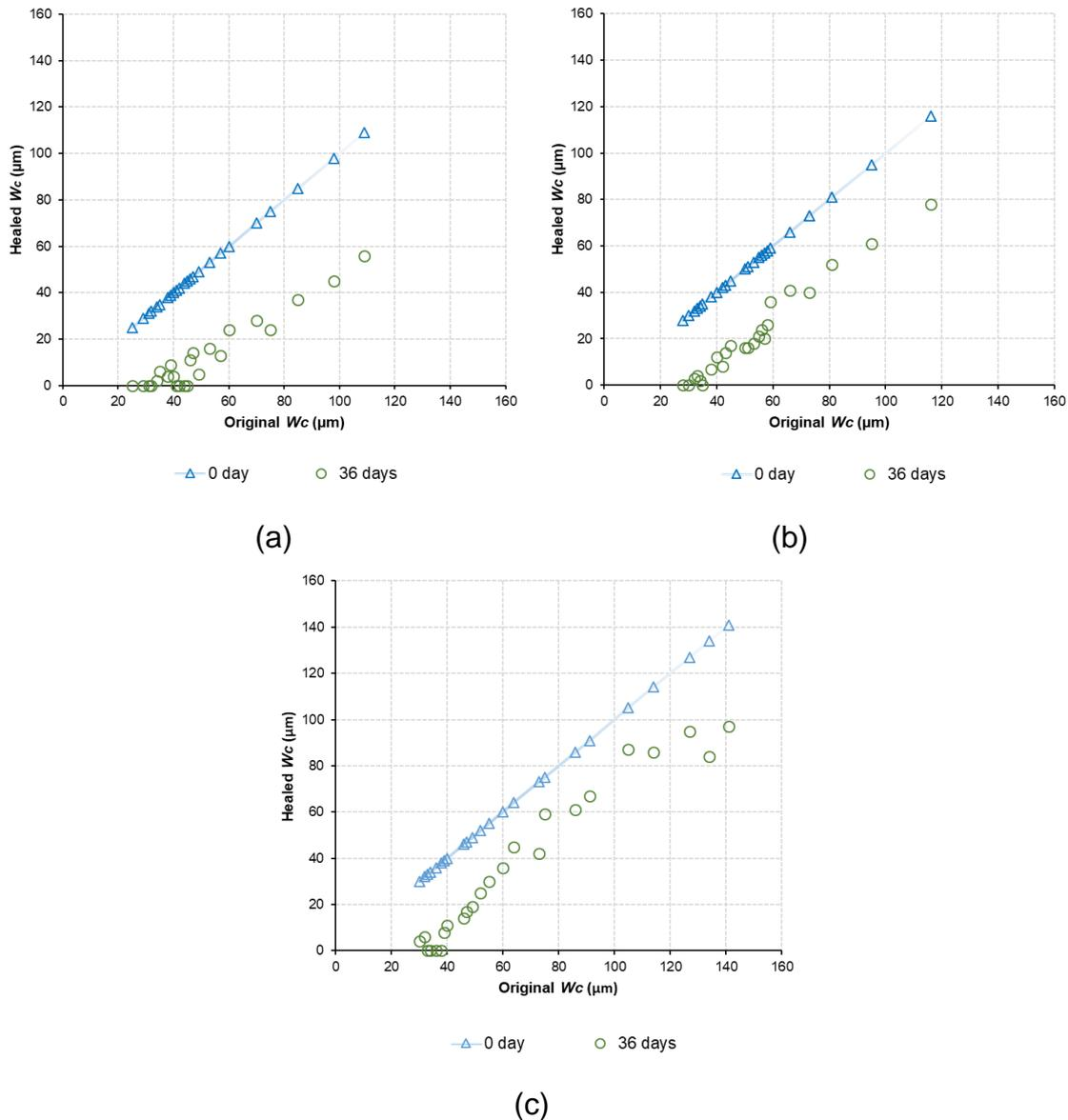
**Fig. 1** Crack width reduction observed on the specimens' surface of: (a) S-C, (b) S-E, and (c) S-S mixtures
